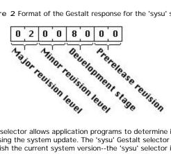
The presence of the 'sysu' Gestalt selector allows application programs to determine if the current installed system software version was established using the system update. The 'sysu' Gestalt selector will only be defined if a system update package was used to establish the current system version--the 'sysu' selector is not defined on machines shipped with System 7.5.3 installed.
